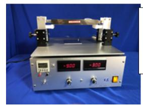
Tungsten wire manual electrification device with a grid electrode timer.
