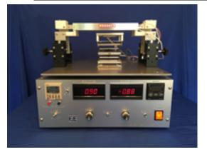
Tungsten wire manual electrification device with a grid electrode. It can be used in various fields such as grid electrode mounting, thermal electret element and micro electret condenser. It is a fully
