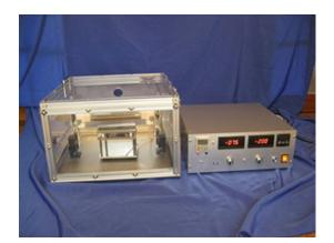
Tungsten wire manual electrification device. It can be used in various fields such as grid electrode mounting, thermal electret element and micro electret condenser. Fully equipped with safety box.
